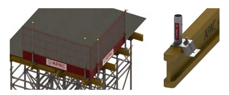
The Timber Beam Clamp is designed to connect H20 beams with the TG Post and TG Barrier. It is adjustable to fit with 40mm & 60mm H20 beams. Compatible with European proprietary timber beam sections.
