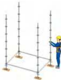
▲ Assembly with base collar can be assembled by even one person.
