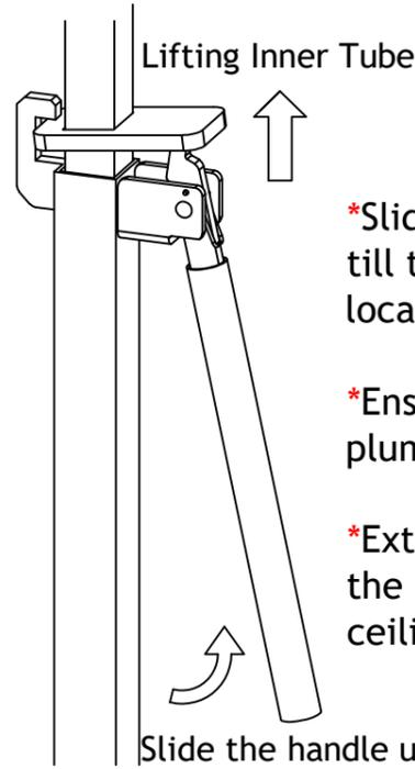
\*Slide the adjustment handle up till the ring is at its desired location
