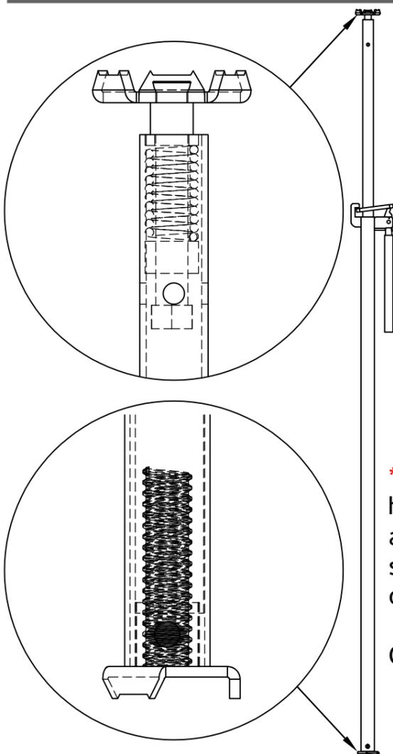
\* Before slide the handle down, the top anchor claw, the spring is free inside of the inner tube
