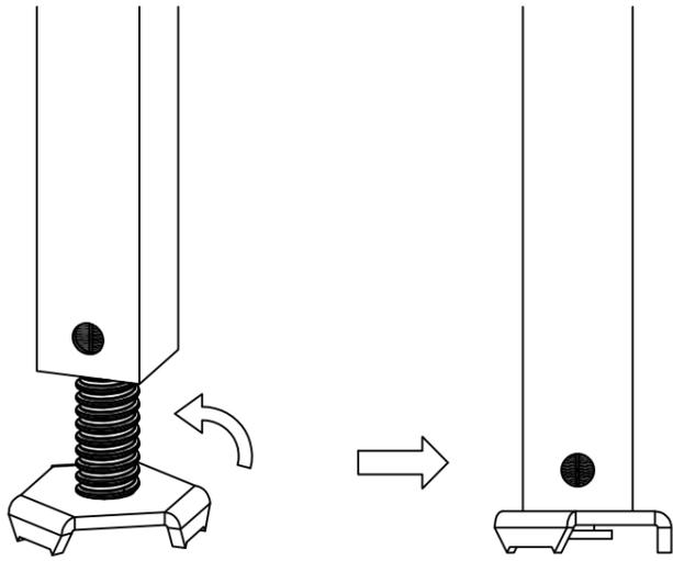
\*Ensure bottom foot is fully screwed into the Compression Post
