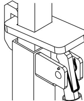
\* The torsion spring will ensure that the handle does not bounce back
