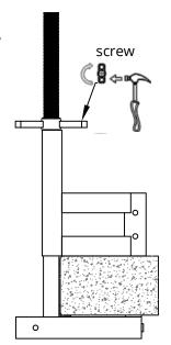
\* Tighten the nut by hand and then hammer it to secure the clamp to the floor
