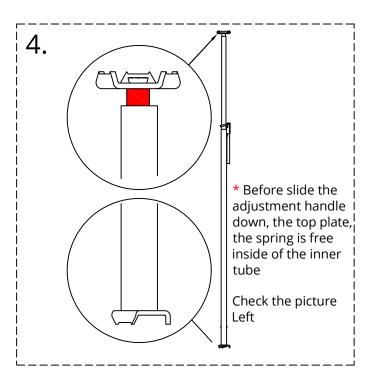
\* When sliding the adjustment handle at Final postion the spring will be compressed then make the top plate come down toward the inner tube \* View the inspection gauge. In the event it is showing any yellow, rotate the post counter clockwise until the RED is no longer visible. Check the right picture \* When dismantle the post, rotate the post clockwise first,then
