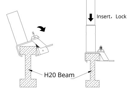
Loosen the butterfly nut and adjust the width
